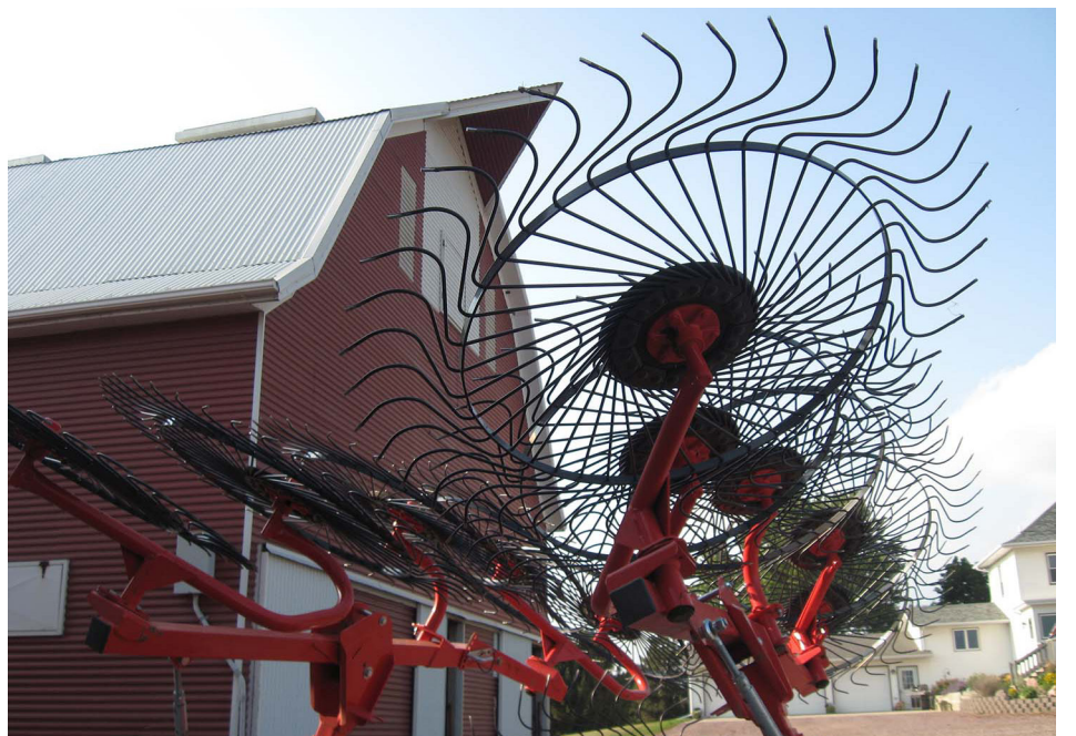
This machine can gather up hay even in the ditches along the roadway to make it easier for the baler to pick it up and make into round hay bales.
