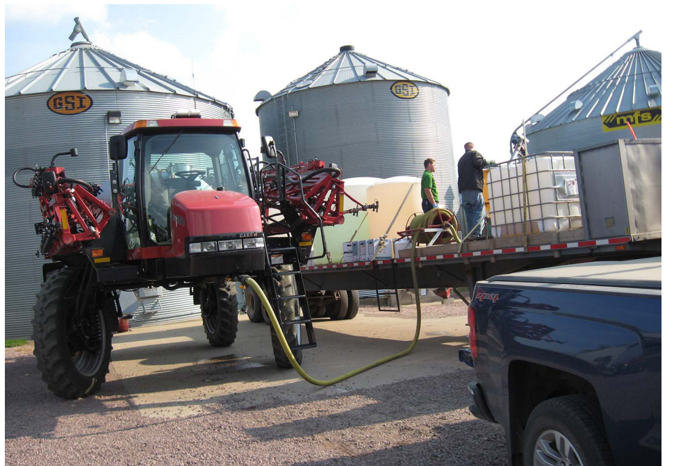
The chemicals are mixed on the flatbed of the Peterbilt and transferred to the sprayer with a hose. The arms of the sprayer extend out twice to spray.
