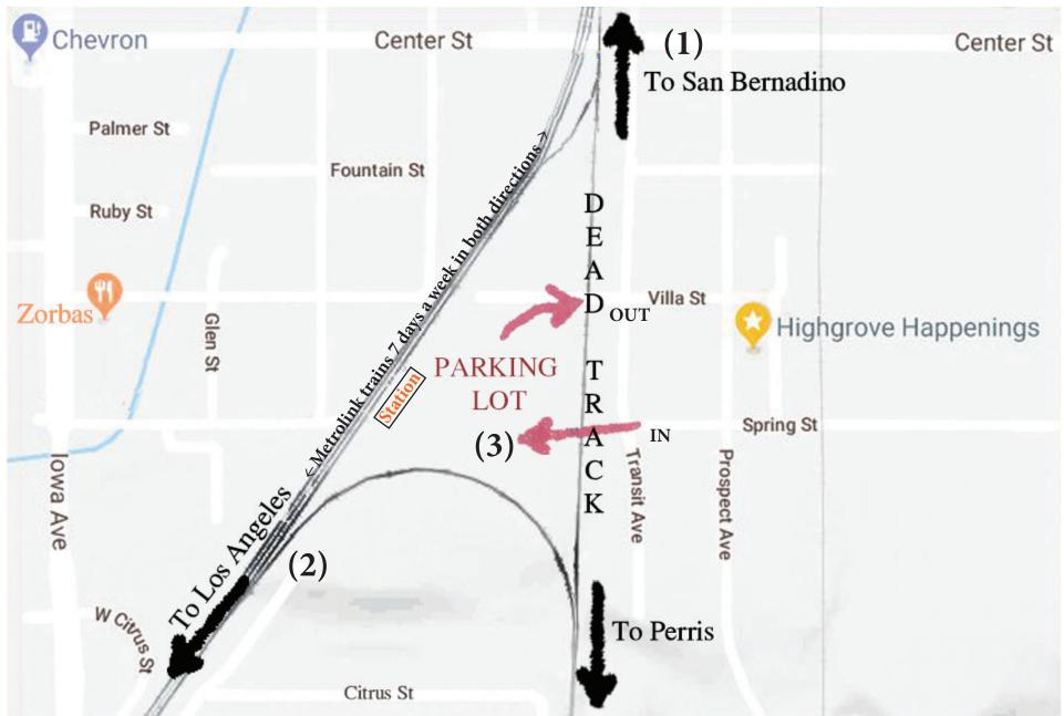
When the new curved track was built to connect the Perris Valley Line track to the BNSF main line for the new Metrolink trains, it also eliminated the freight train traffic on the straight track between Main Street and the east end of the curved track where it connects to the Perris Valley Line track. Today, there are no Metrolink trains or freight trains on this dead track.
