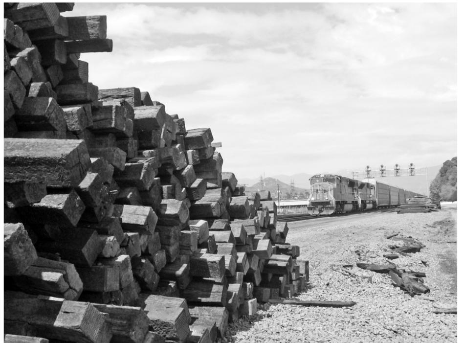
New railroad ties have been replaced in the track through Highgrove. Here is a westbound Union Pacific train going through Highgrove passing by some of the railroad ties used as part of the maintenance program. The UP, BNSF, Amtrak and Metrolink use the tracks through Highgrove.
